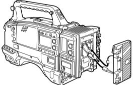
**5** Use the screws to screw the battery mount onto the camera adapter.
