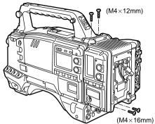
4 Connect the connectors on the battery mount to the connectors on the camera adapter.
